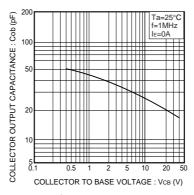
Fig.5 Collector output capacitance vs. collector-base voltage
