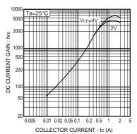
Fig.2 Grounded emitter propagation Fig.3 DC current gain vs. collector current characteristics
