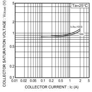
Fig.4 Collector-emitter saturation voltage vs. collector current
